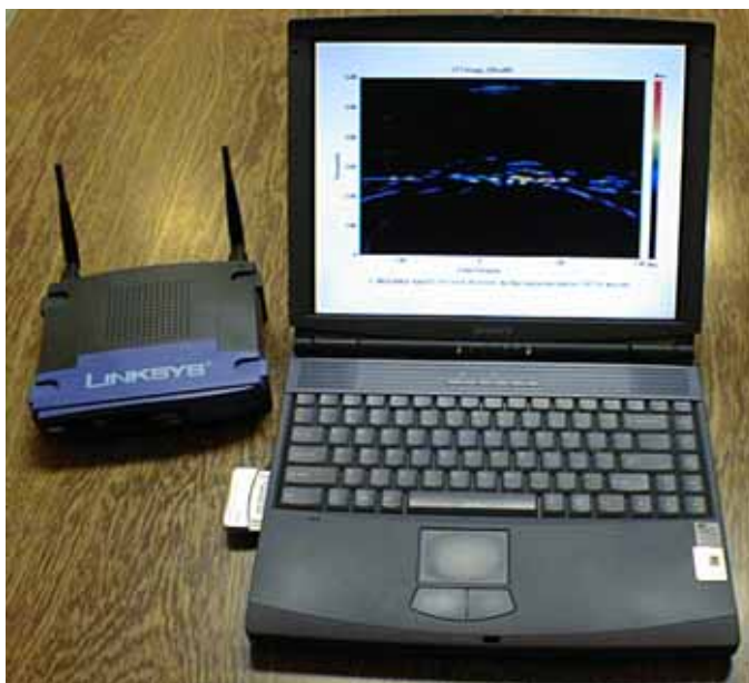
Figure 3 - Display/fusion node and wireless radar sensor node.
