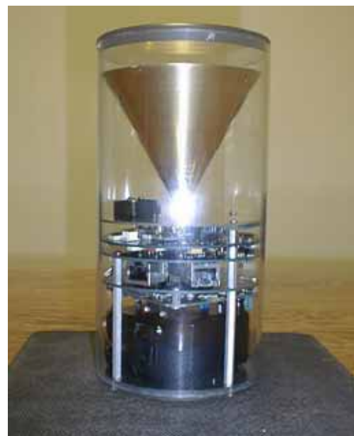
Figure 3 - Display/fusion node and wireless radar sensor node.
